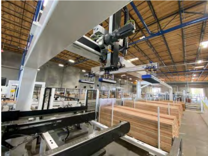
Photo 17- Entekra LLC fully automated off-site construction
