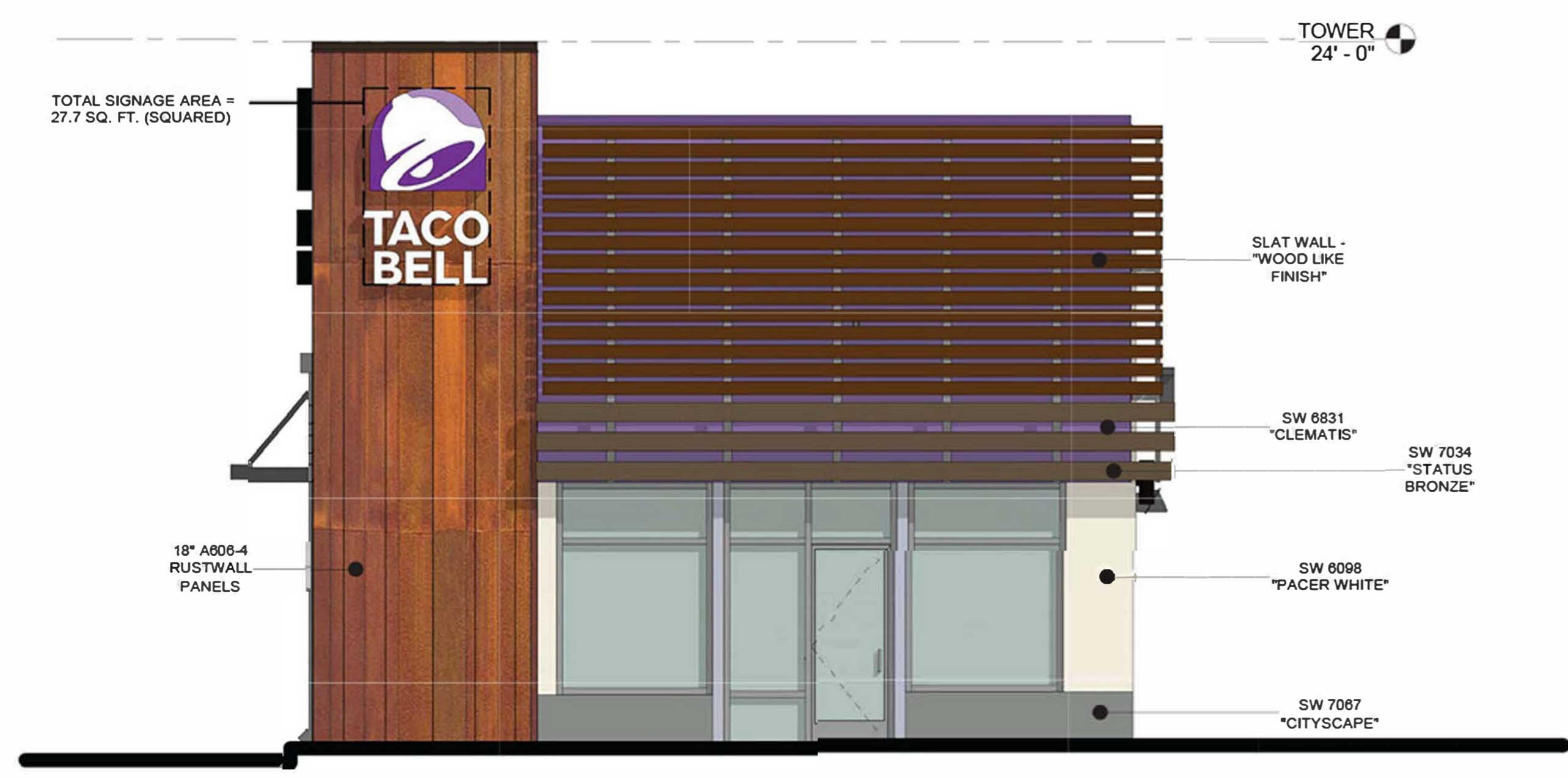
SOUTH ELEVATION - FRONT SC: 1/4"=1'-0" 9
