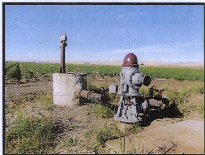
Figure 9: Well 6/8-20G is maintained well, but has no engine, thus is not in use.
