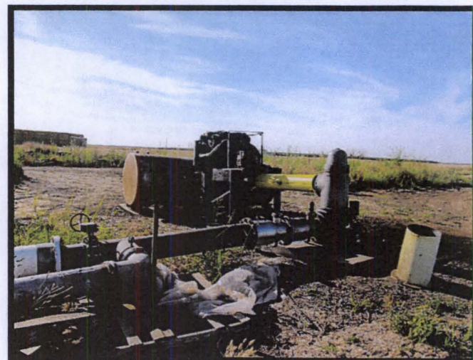
Figure 11: Well 6/8-8J is being used to irrigate fields, connected to a diesel engine.
