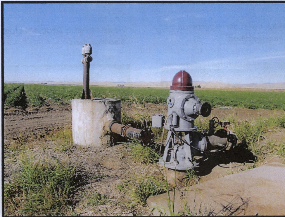
Figure 12: Well 6/8-20G has a new pump and could be operational if a diesel engine was attached.
