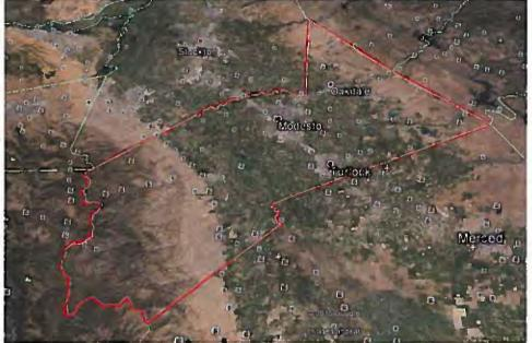
Orthoimagery Resolution: Horizontal Accuracy of Imagery: Imagery Radiometry: Projection and Datum: 6-inches ASPRS Class I at 1"=100' 3-band, 8-bits per channel, RGB California State Plane Coordinate System, Zone 3, NAD83 (2011), US Survey Foot TBD
