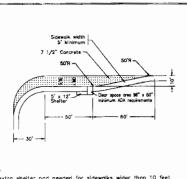
NOTES: 1. No extra shelter pad needed for sidewalks wider than 10 feet. Shelter pad and shelters must be wide enough to meet ADA requirements 4.0" x 3.0" clear floor area within shelter
